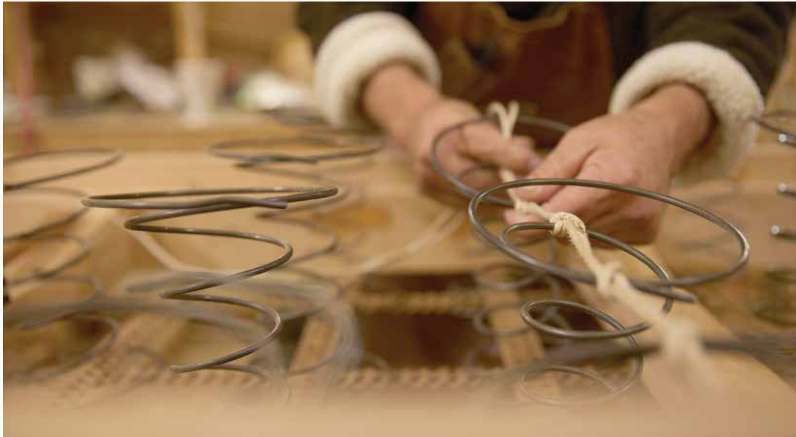
8-way hand tied construction
